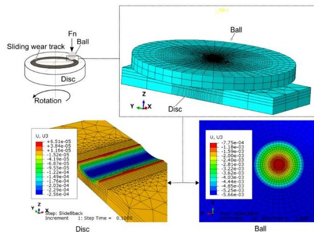
Figure 1: Summary of FE model and wear profiles on the ball and disc surfaces after reduction of artificial roughening
