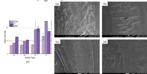
Figure 1: (a) wear track of E-48, (b) E-49, (c) E-50, (d) E-51, (e) wear loss after hydrogen exposure.
