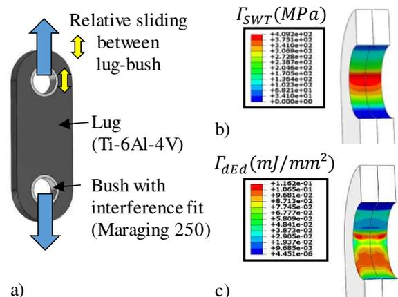
Figure 1 : Lug-bush assembly (a), distribution of SWT (b) and dEd (c) along a lug bore
