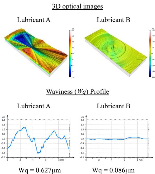
Figure 1: Surface waviness of two tappets from two different test lubricants
