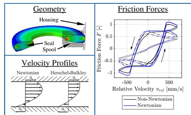
Figure 1: Investigated geometry, velocity profiles and calculated friction forces depending on chosen model.
