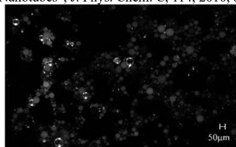
Figure 1: Photograph of fluorinated particles polymerized by proposed method
