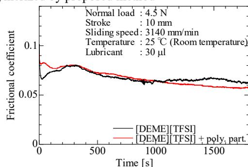
Figure 2: Friction behavior of [DEME][TFSI] and [DEME][TFSI] + fluorinated polymer particles.
