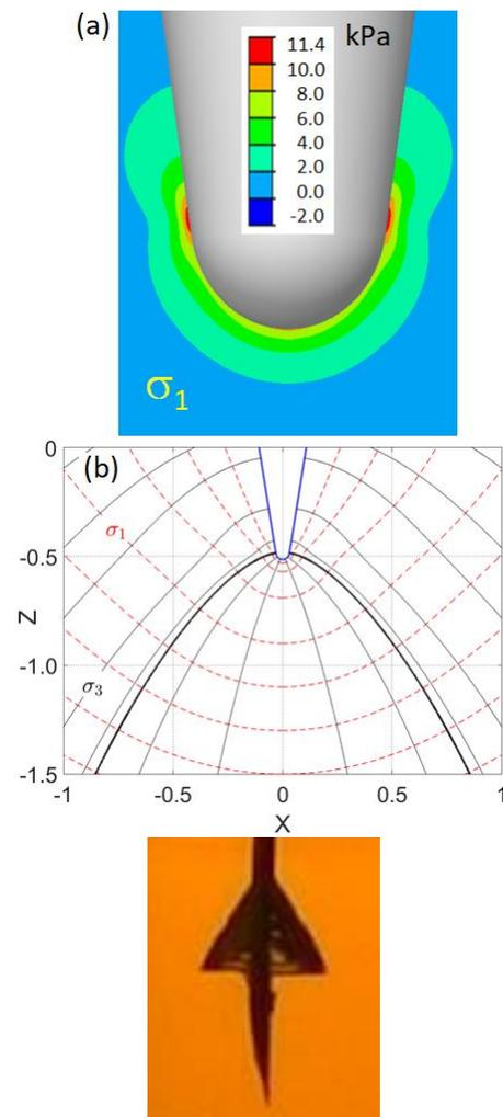
Figure 2: (a) Maximum principal stress ( $\sigma_1$ ) contour. (b) Maximum ( $\sigma_1$ ) and minimum ( $\sigma_3$ ) principal stress trajectories. (c) Deep penetration of needle induced cone crack in a soft hydrogel.
