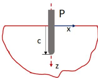
Figure 1: Schematic of rigid spherical tip indenter at a point interior in a semi-infinite solid.
