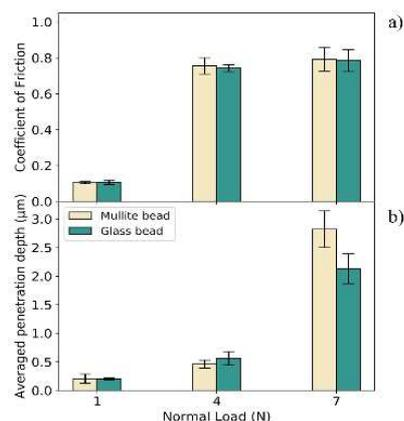
Figure 1: The effect of normal load on a) friction coefficients and on b) averaged penetration depth, for mullite and glass beads.
