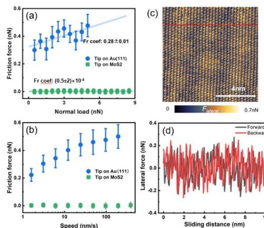
Figure 1: Friction characterizations of MoS<sub>2</sub> and Au(111) surfaces.
