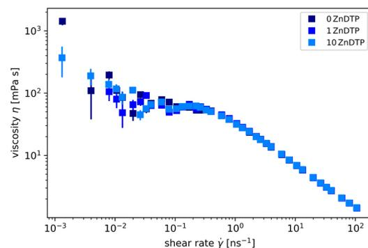
Figure 2: Comparison of shear thinning curves of PAO4 with 0, 0.5 or 5 mass percent ZnDTP as additives in systems with a pressure of 250 MPa.
