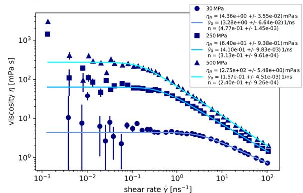
Figure 1: Comparison of shear thinning curves of PAO4 at 30 MPa (circles), 250 MPa (squares) and 500 MPa (triangles) with fits of the Carreau equation (blue lines).
