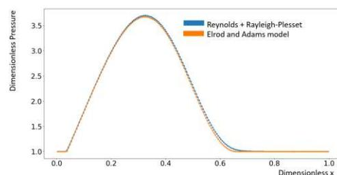
Figure 1: Pressure in the bearing mid-plane
