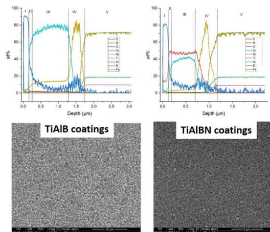
Figure 1: GDOES depth profile and SEM images of the surface of selected TiAlB and TiAlBN coatings.
