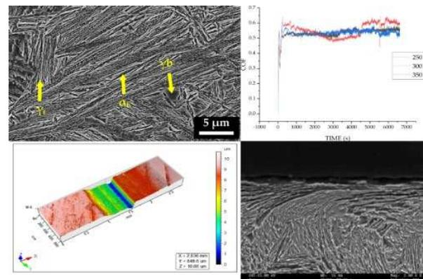
Figure 1: Microstructure before and after wear tests, friction coefficient variations with sliding distance, 3D isometric view of the wear track.
