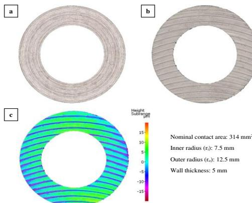
**Fig. 1.** Optical profilometry images of (a) the smooth and (b) rough specimens, and (c) 3D surface topography of the rough surface.
