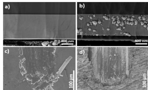
Figure 1: Cross sections and wear tracks of a,c) Ti-rich, b,d) Ag-rich Ti-Ag films;
