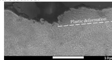
Figure 1: Cross-section of cracks and micropits.
