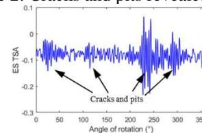
Figure 3: Cracks and pits revealed in ES.
