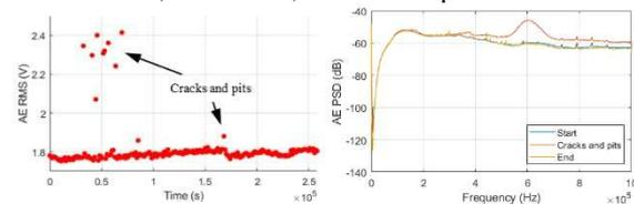
Figure 2: Cracks and pits revealed in AE.
