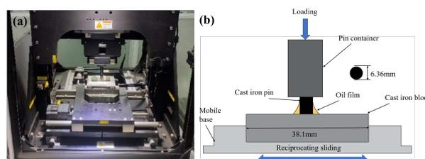
Figure 1: reciprocating sliding test apparatus: (a) R-tec-tribo-tester; (b) schematic view of the experimental process.
