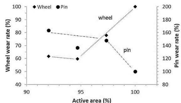
Figure 2: Pin and disc wear rate (%) as a function of the wear track active area (%).
