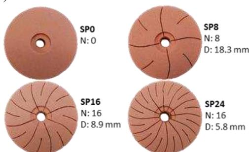
Figure 1: Produced grinding wheels. N - number of grooves (width: 0.5 mm, depth: 3 mm) and D - distance between the grooves.
