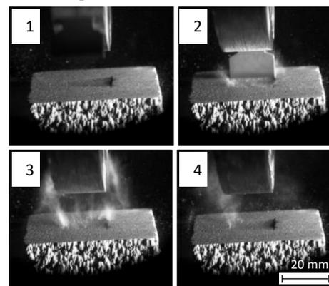
Figure 1. Images series showing compaction after a strike of the blade
