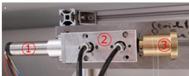
Figure 2: Bearing friction measurement components: Driving motor (1), air bearing (2), bearings under test (3).
