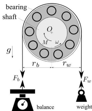
Figure 1: Measurement principle using a balance to register friction force and a known weight to define the radial load. The axial preload is defined by a preloaded spring. Note:  $r_w \neq r_b$
