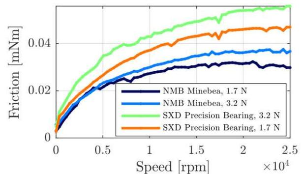
Figure 3: Friction measurements on two different ball bearings (DIN 625-1) at room temperature, dimensions: 6 mm x 2 mm, lubricant: Multemp SRL.
