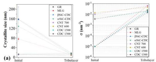
Figure 1: Quantification of defects before and after the tests (a) Crystallite size (b) Point defect density.
