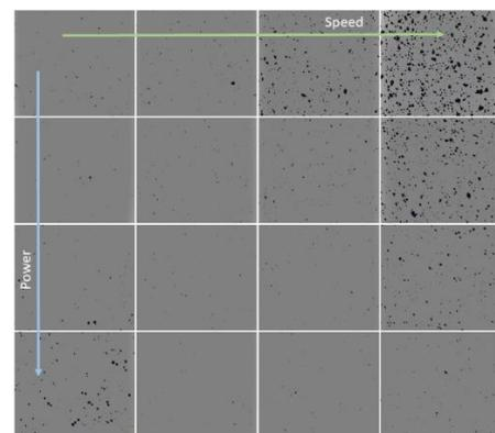
Figure 1: Top surface porosity of prepared samples.
