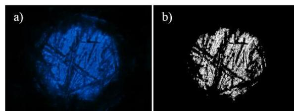
Figure 1: (a) Raw microscope sample image; (b) processed real contact area image.
