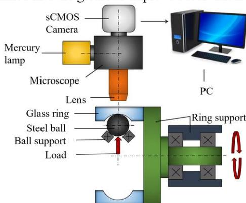
Figure 1: Schema of experimental apparatus.
