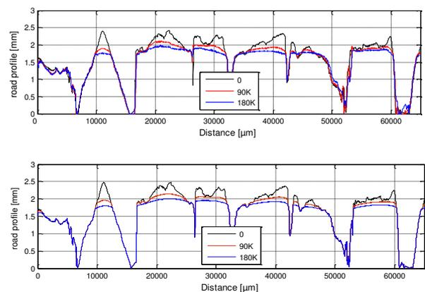
Figure 1: Direct comparison between the experiment (top) and simulation (bottom) of texture evolution of one of the pavement specimens made with limestone aggregates (K = 1000)
