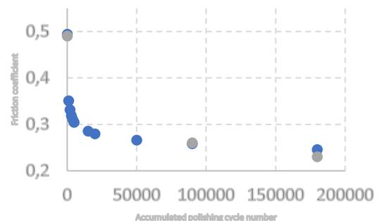
Figure 2: Direct comparison between the experiment (Blue dots) and simulations (Grey dots) of friction coefficient evolution of one of the pavement specimens made with limestone aggregates
