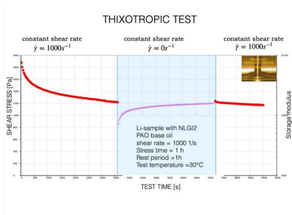
Fig.1: Example for the test procedure
