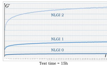
Fig.2: Evolution of the storage modulus for different grease samples during the rest period
